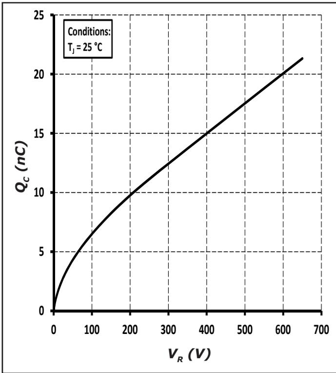
Figure 3. Total Capacitance Charge vs. Reverse Voltage
