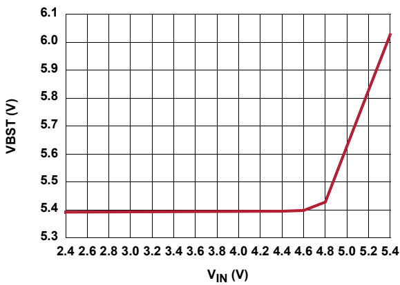
FIGURE 8. VBST, V_{IN} HEADROOM TRACKING, V_{BST} = 5.4\text{V}
