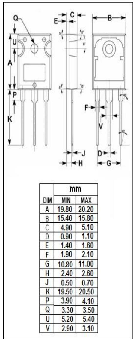
**isc N-Channel MOSFET Transistor****R6030ENZ1****ELECTRICAL CHARACTERISTICS** $T_c=25^\circ\text{C}$  unless otherwise specified
