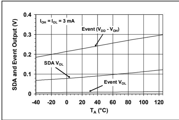
**FIGURE 2-7:** Event and SDA  $V_{OL}$  vs. Temperature.
