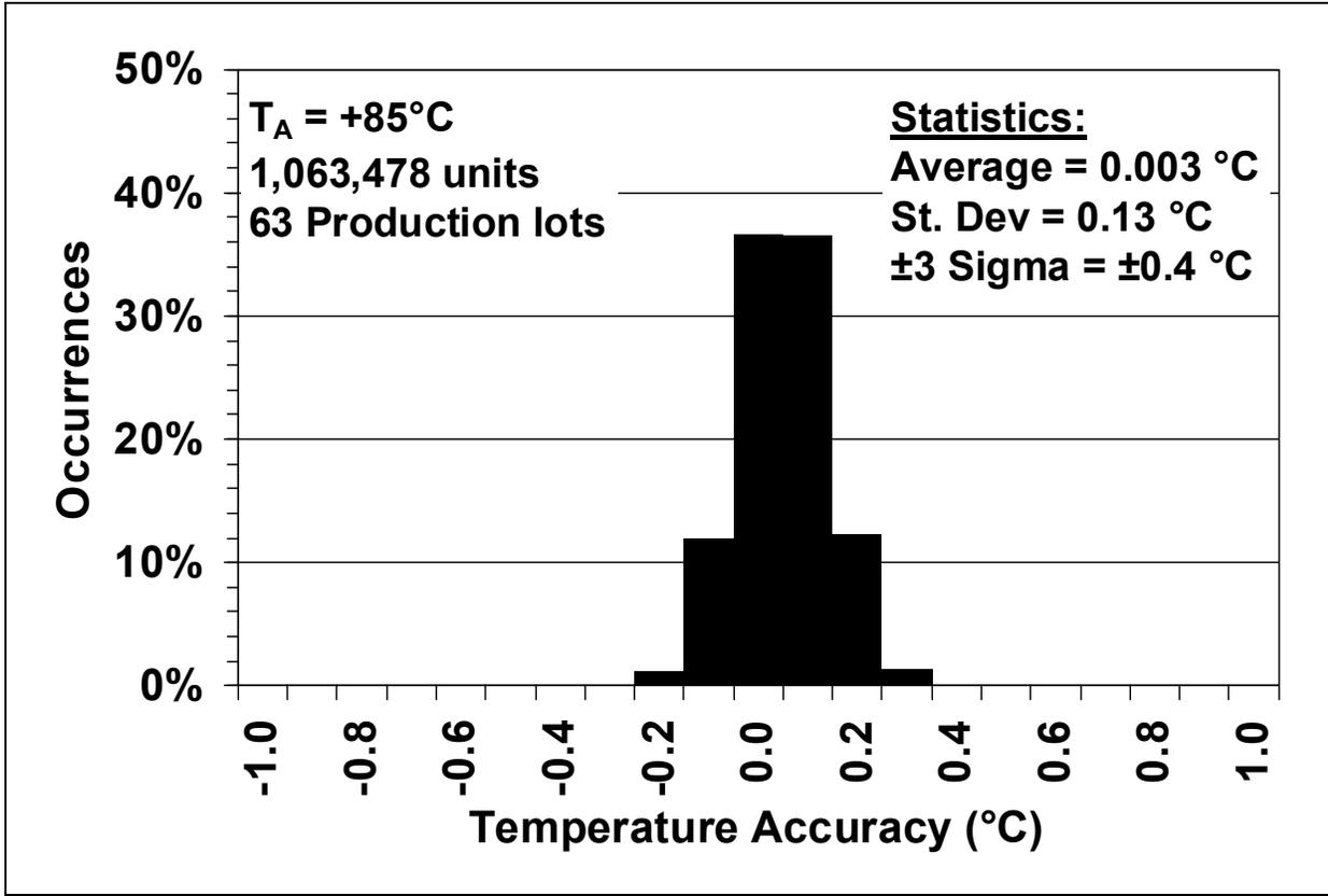
**Note:** This accuracy data from the production system represents the typical accuracy performance of the MCP98242 Memory Module Temperature Sensor. The MCP98242 production methodology is also used for the MCP9843/98243 to achieve the same typical accuracy performance.
