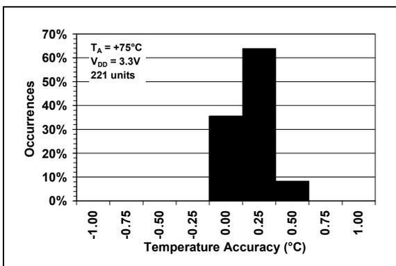
**FIGURE 2-3:** Temperature Accuracy Histogram,  $T_A = +75^{\circ}C$ .
