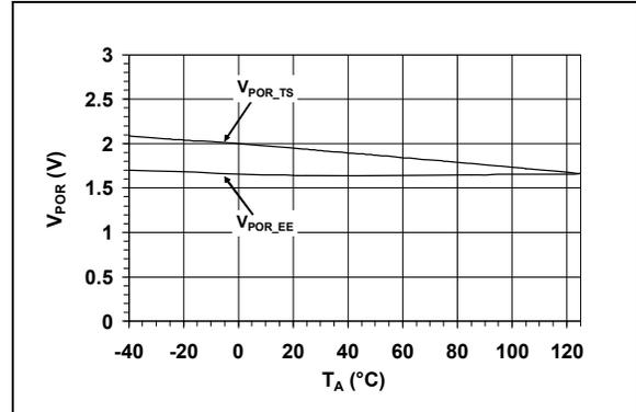
**FIGURE 2-6:** Power-on Reset Threshold Voltage vs. Temperature.
