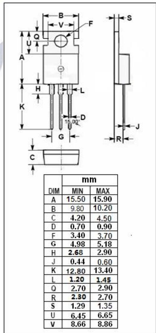
**isc N-Channel MOSFET Transistor****60N05-16****• ELECTRICAL CHARACTERISTICS ( $T_c=25^\circ\text{C}$ )**
