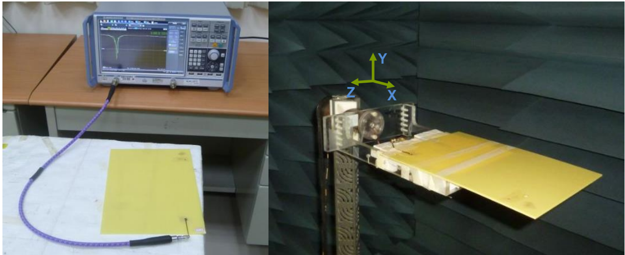
Figure 1. Impedance measurements (left side) and peak gain, efficiency and radiation pattern measurements (right side).
