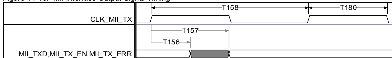
Figure 14-15. MII Interface Output Signal Timing
