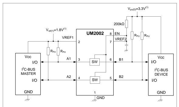
(1) The applied voltages at  $V_{\text{ref(1)}}$  and  $V_{\text{pu(D)}}$  should be such that  $V_{\text{bias(ref)(2)}}$  is at least 1 V higher than  $V_{\text{ref(1)}}$  for best translator operation.
