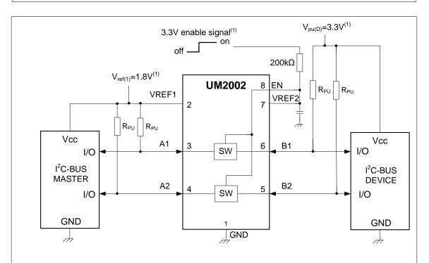
(1) In the Enabled mode, the applied enable voltage  $V_{I(EN)}$  and the applied voltage at  $V_{ref(1)}$  should be such that  $V_{bias(ref)(2)}$  is at least 1 V higher than  $V_{ref(1)}$  for best translator operation.
