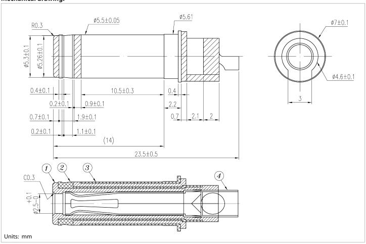
tolerance X:  $\pm 0.5 \, \text{mm}$  .X:  $\pm 0.3 \, \text{mm}$  .XX:  $\pm 0.05 \, \text{mm}$  applicable unless otherwise indicated in specification or on drawings
