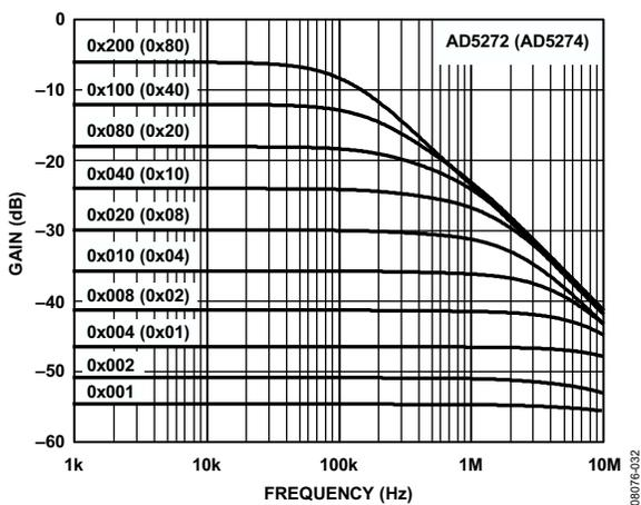
Figure 26. 50 kΩ Gain vs. Code vs. Frequency
