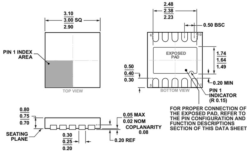
Figure 50. 10-Lead Frame Chip Scale Package [LFCSF\_WD]
