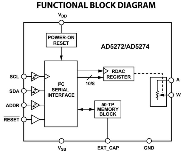
The AD5272/AD5274 device wiper settings are controllable through the I<sup>2</sup>C-compatible digital interface. Unlimited adjustments are allowed before programming the resistance value into the 50-TP memory. The AD5272/AD5274 do not require any external voltage supply to facilitate fuse blow and there are 50 opportunities for permanent programming. During 50-TP activation, a permanent blow fuse command freezes the wiper position (analogous to placing epoxy on a mechanical trimmer).
