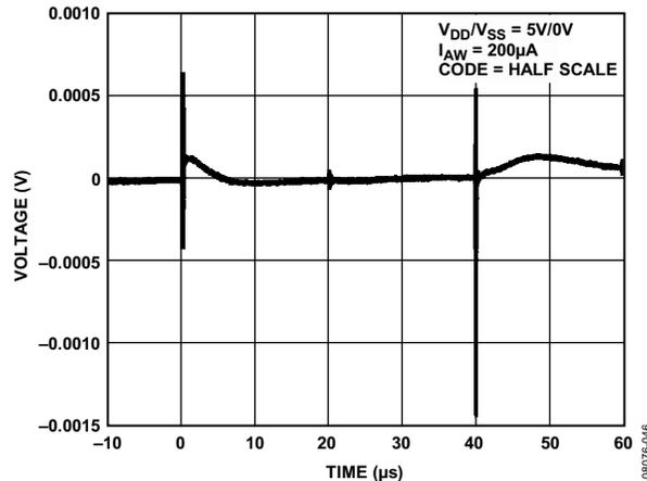
Figure 34. Digital Feedthrough
