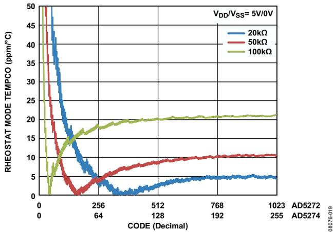
Figure 24. Tempco  $\Delta R_{WA}/\Delta T$  vs. Code
