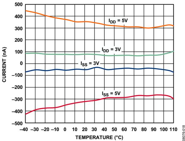
Figure 20. Supply Current ( $I_{DD}$ ,  $I_{SS}$ ) vs. Temperature
