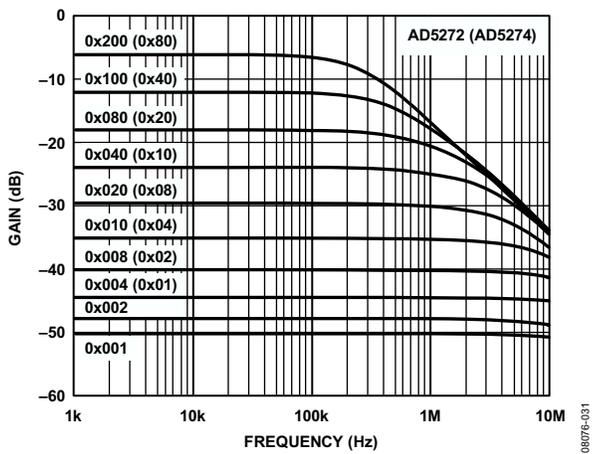
Figure 25. 20 kΩ Gain vs. Code vs. Frequency
