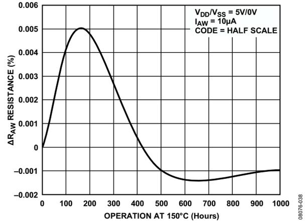
Figure 37. Long-Term Drift Accelerated Average by Burn-In
