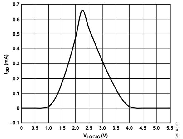
Figure 23. Supply Current ( $I_{DD}$ ) vs. Digital Input Voltage
