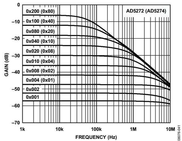
Figure 28. 100 kΩ Gain vs. Code vs. Frequency
