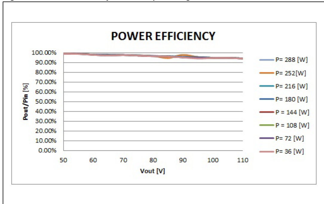
Figure 13. MPPT efficiency versus output voltage
