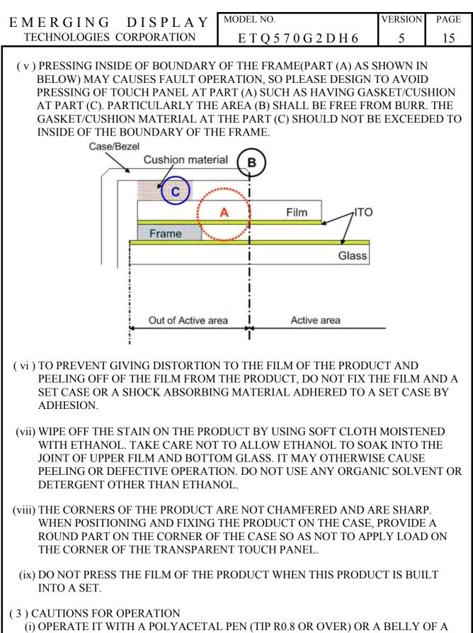
1) OPERATE IT WITH A POLYACETAL PEN (TIP R0.8 OR OVER) OR A BELLY OF A FINGER WITHOUT APPLYING EXCESSIVE LOAD. NEVER USE ANY MECHANICAL PENCILS, BALL POINT PENS AND HARD FINGERTIPS WHOSE TIP IS HARD FOR INPUT, OTHERWISE MALFUNCTIONS MAY RESULT.
