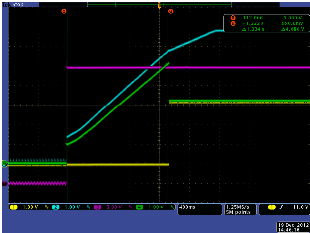
Figure 6. TSS721A Startup ( C_{STC} = 220 \mu\text{F} , 1 Unit Load, BSS84L, external load of 8 k \Omega ) (purple = BUSL1, blue = STC, yellow = VDD, green = PFb)
