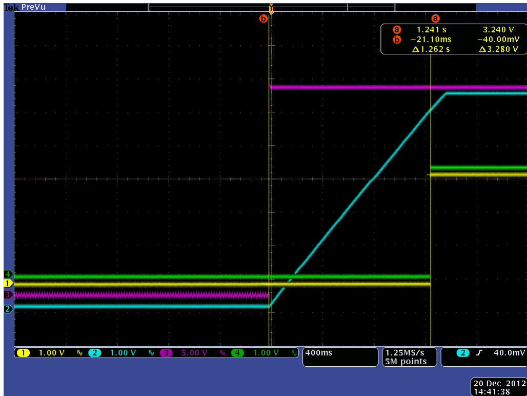
Figure 3. NCN5150 Startup ( C_{STC} = 220 \mu F , 1 Unit Load, no STC transistor) (purple = BUSL1, blue = STC, yellow = VDD, green = PFb)
