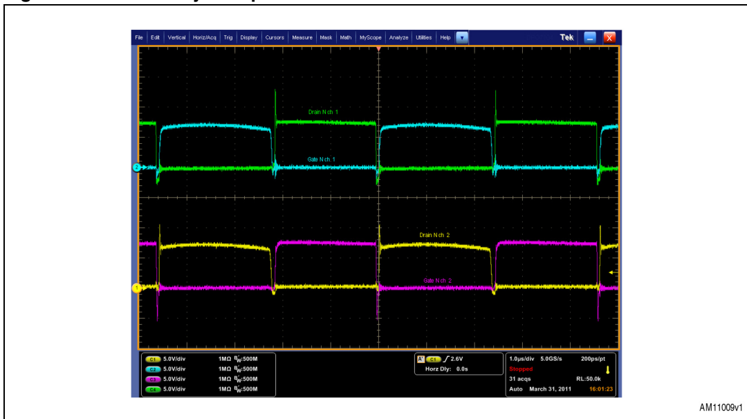
Figure 12. Secondary-side power MOSFET waveforms at 16 A load
