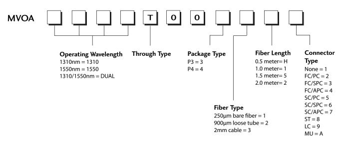
\* The tolerance of fiber length is +/-0.1m.
