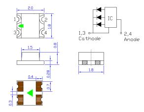
Notes: 1. All dimensions are in millimeters; 2. Tolerance is  $\pm$  0.15 mm unless otherwise noted.
