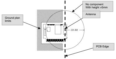
Ideally, the module can be placed in edge of the PCB.
