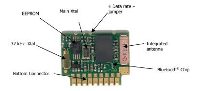
Pin-out All connections are located on the A<sup>RF32</sup> bottom connector:
