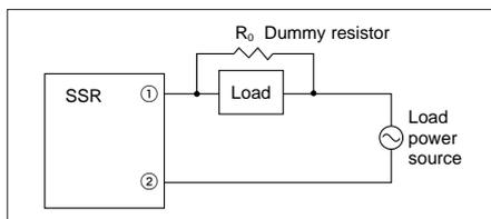
In case the dummy resistor is not used, keep in mind that the residual voltage becomes as follows:
