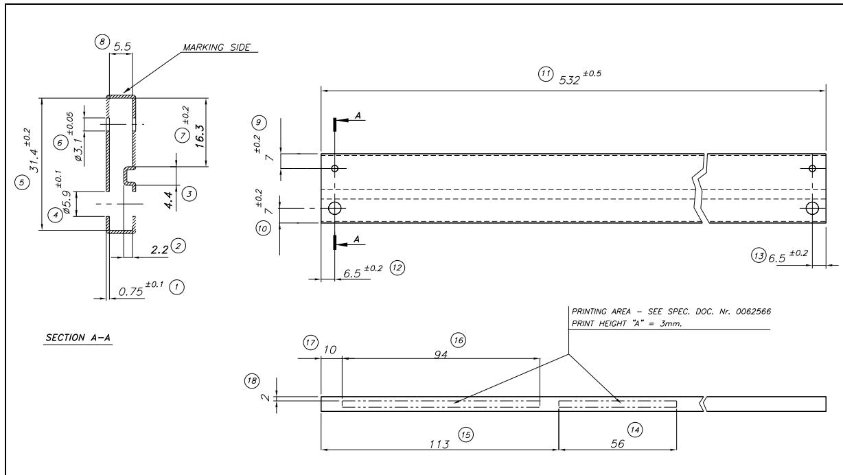
**Tube for TO-220 (single gauge) (mm.)**
