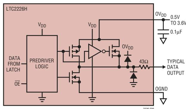
Figure 9. Digital Output Buffer
