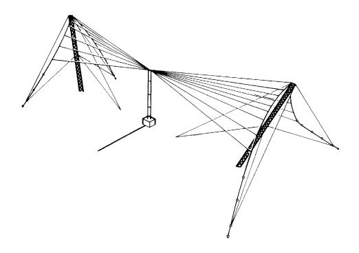
The 1765 antennas require no tuning or resistive loading circuitry. This permits complete compatibility with multichannel fixed-tuned radios as well as frequency agile, synthesized HF radio equipment. Elimination of the antenna coupler maximizes the power output of the antenna/transmitter, resulting also in a significant improvement in communication reliability through the reduction of maintenance and/or repair.
