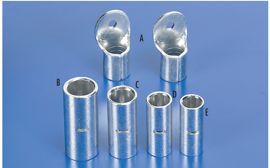
Large Brazed-Seam Terminals: A = 400 MCM Wire Gauge Large Brazed-Seam Splices: B = 500 to 600 MCM Wire Gauge, C = 350 to 450 MCM Wire Gauge D = 300 to 350 MCM Wire Gauge, E = 250 to 300 MCM Wire Gauge
