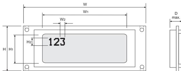
**REFLECTIVE** : Using ambient light for display visibility, they are ideal for energy saving applications.
