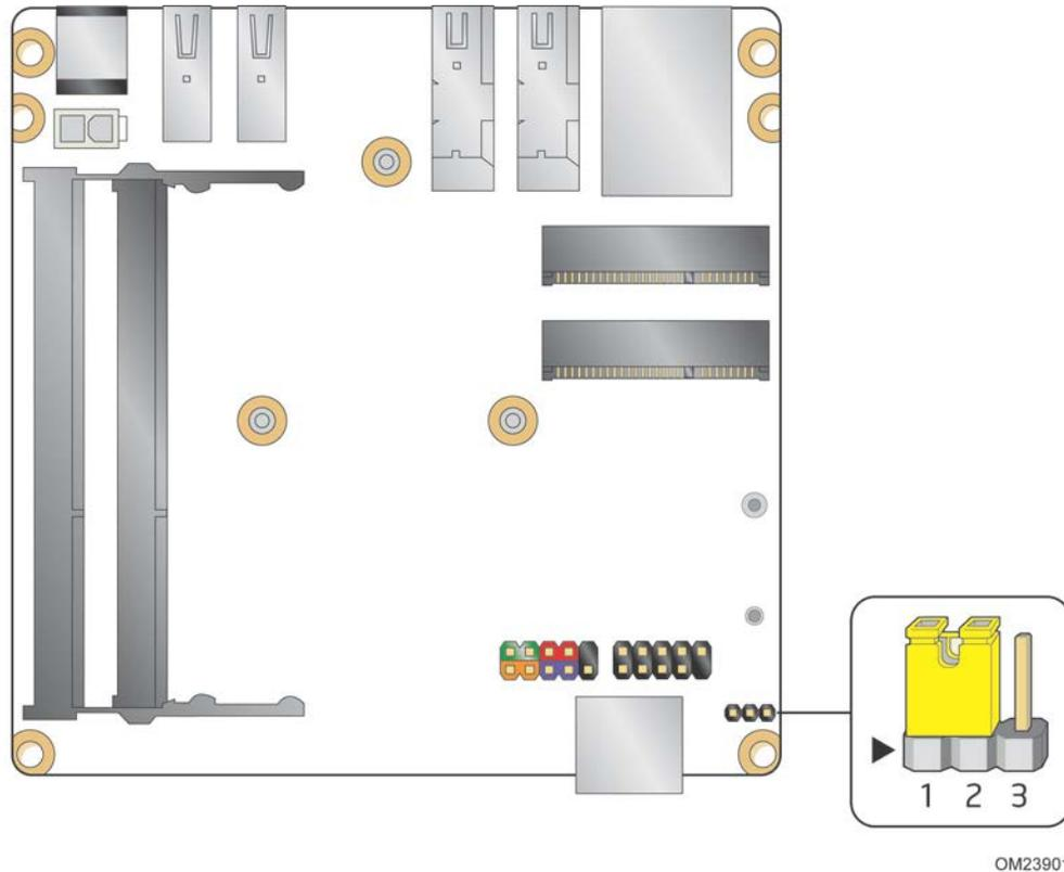
**Figure 13. Location of the BIOS Configuration Setup Jumper**
