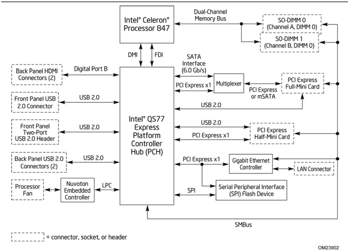
Figure 3. Block Diagram
