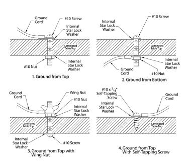
B. 3M<sup>™</sup> Wrist Strap Grounding System 3042: This is an accessory product that can be permanently mounted to a laminate-covered workbench. It is designed to allow the operator(s) at that bench to connect wrist strap cords to the same ground to which the laminate benchtop is connected. The 3M Grounding System is a small module containing two banana jacks, side-by-side, which will accept the banana plugs on the ground cords of standard static control wrist straps.
