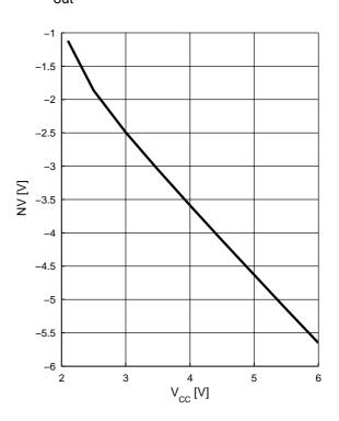
Output Voltage, AC-coupled,  $V_{CC} = 3 \text{ V}, I_{OUT} = 0 \text{ mA}, C_{OUT} = 100 \text{ nF}$  Output Voltage, AC-coupled,  $V_{CC}$  = 3 V,  $I_{OUT}$  = 3 mA,  $C_{OUT}$  = 100 nF
