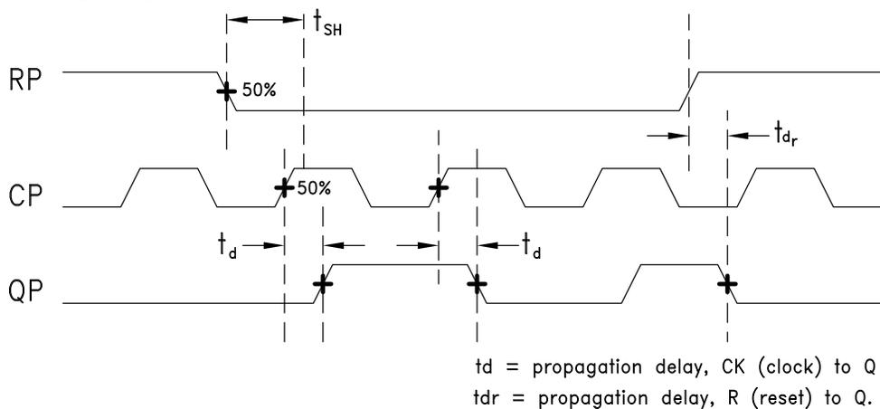
$t_d$  = propagation delay, CK (clock) to Q
