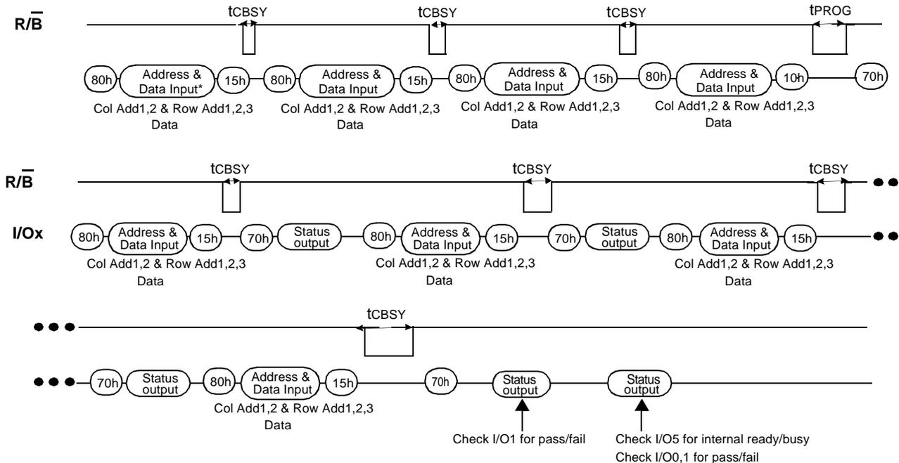
**NOTE :** Since programming the last page does not employ caching, the program time has to be that of Page Program. However, if the previous program cycle with the cache data has not finished, the actual program cycle of the last page is initiated only after completion of the previous cycle, which can be expressed as the following formula.
