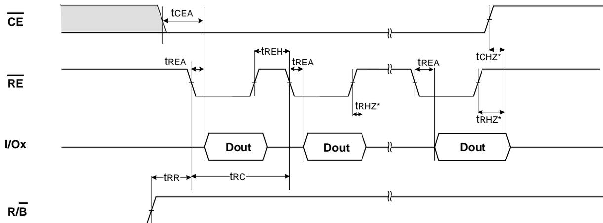
NOTES : Transition is measured  $\pm 200\text{mV}$  from steady state voltage with load.
