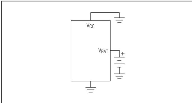
图5. 单电源(V<sub>BAT</sub>)
