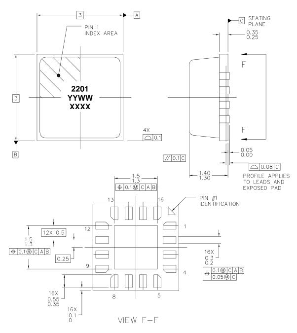
This package is lead-free/RoHS-compliant. The package base is Aluminum Nitride and the plating material on the leads is gold over nickel (Au-Ni). This package is compatible with both lead free and tin-lead soldering processes. The lid is plastic.
