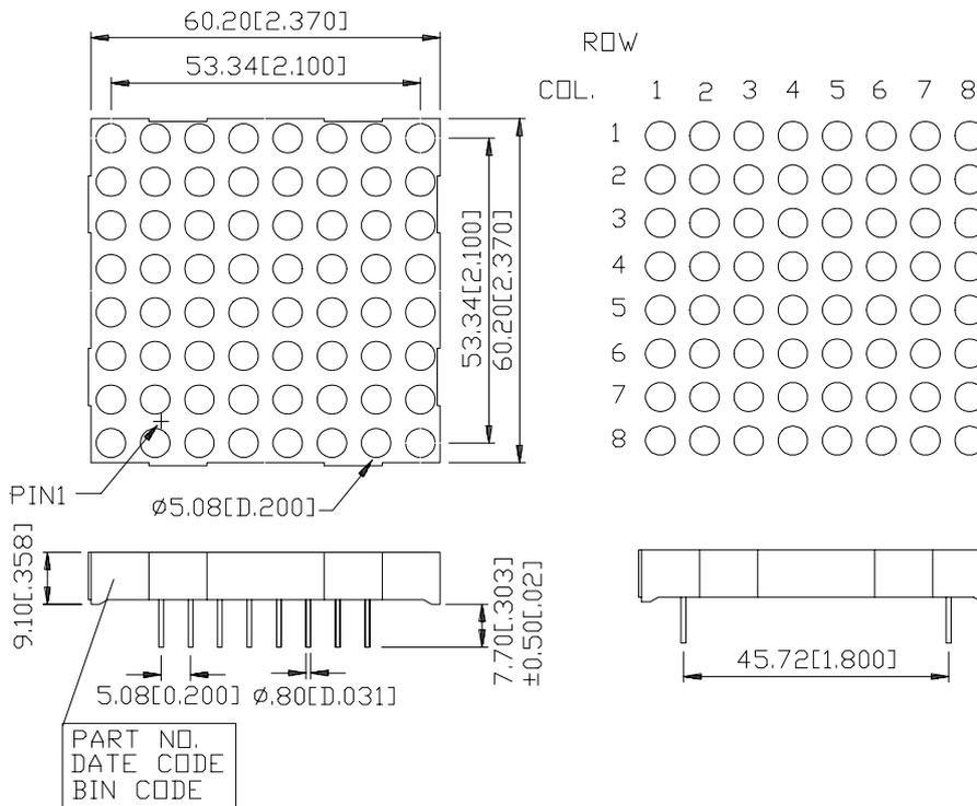
NOTES: All dimensions are in millimeters. Tolerance is  $\pm 0.25$  mm (0.01") unless otherwise noted.
