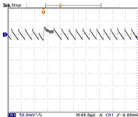
LLM Output Ripple: V_{IN} = 5.0V , V_{OUT} = 3.0V , I_{OUT} = 0.1A , C_{IN} = 22\mu F , C_{OUT} = 2 \times 47\mu F/1206
