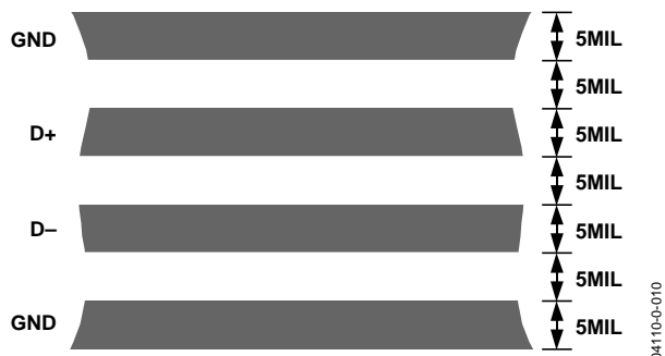
Figure 24. Typical Arrangement of Signal Tracks
