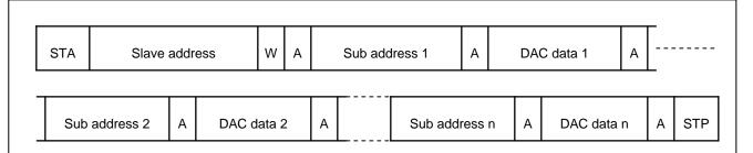
After the Start condition, the transmitting IC accesses the slave IC by Slave address, and transmits the data to each channel by two bites (Sub address and DAC data).
