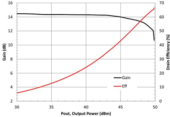
**Gain/ Efficiency vs. Pout, f = 2140MHz**
