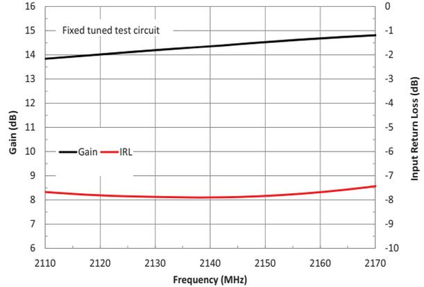
**Gain/IRL vs. Frequency, Pout = 49.5dBm**
