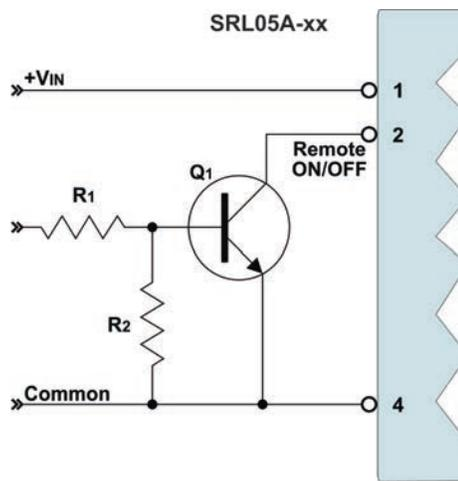
These units include an active high On/OFF control input. The unit is "ON" if the input to the control pin (pin 2) is high; or if the pin is left open (or floating). The signal level of the control input is referenced to ground. A recommended drive circuit for the control pin is shown at left. The resistors R1 & R2 have been added to help reduce possible false triggering of the control input due to leakage currents.
