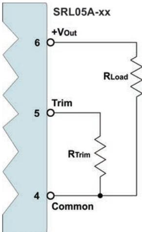
The output voltage level of the **SRL05A** series is adjustable over a wide range by the simple addition of an external resistor. This trim resistor is connected between the circuit common and the trim input (pin 5), as shown in the diagram above.
