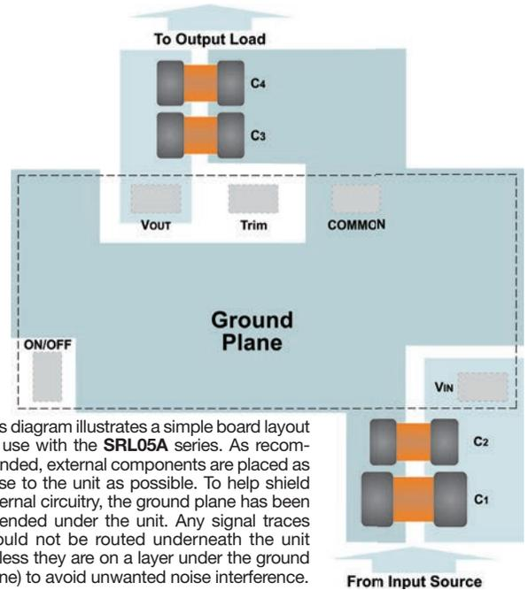
This diagram illustrates a simple board layout for use with the SRL05A series. As recommended, external components are placed as close to the unit as possible. To help shield external circuitry, the ground plane has been extended under the unit. Any signal traces should not be routed underneath the unit (unless they are on a layer under the ground plane) to avoid unwanted noise interference.
