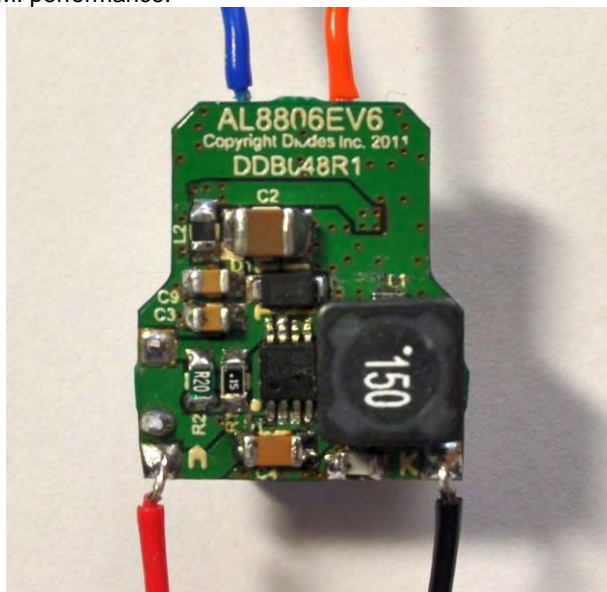
Figure 8. AL8806EV6 evaluation board (Top)
