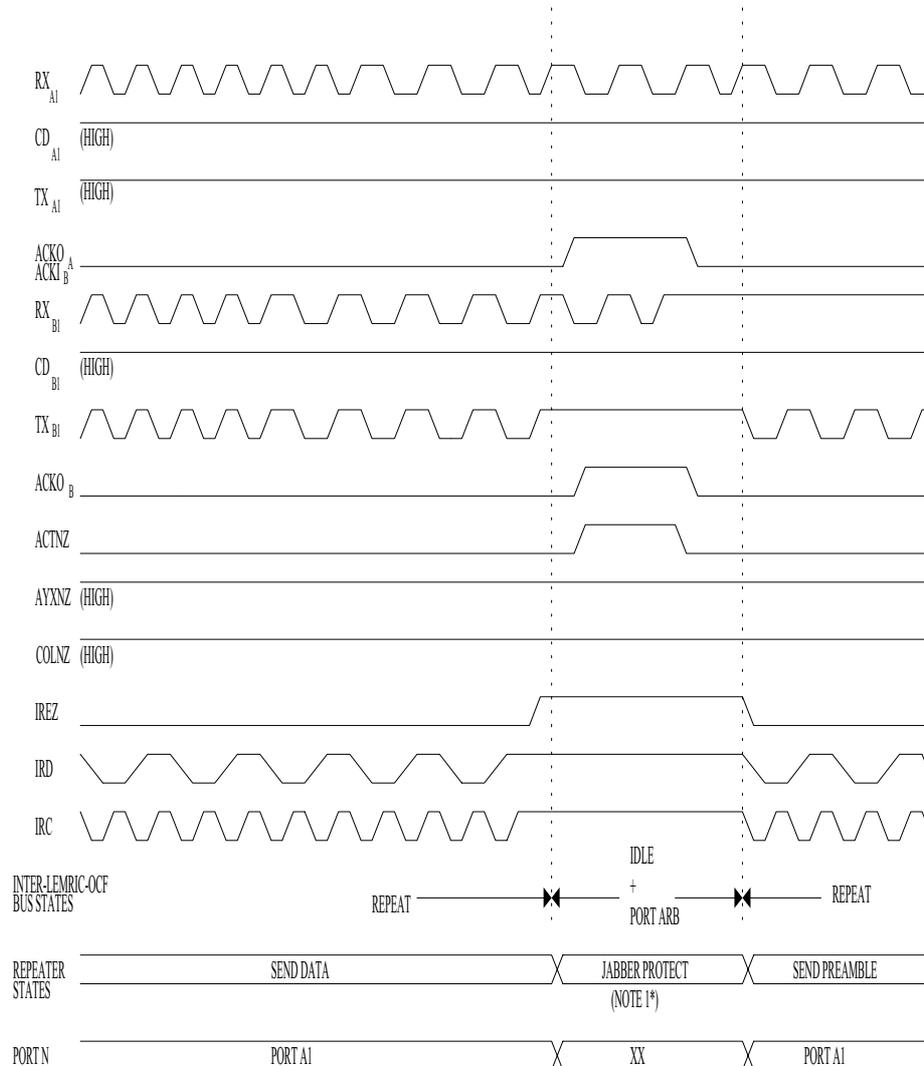
Note 1: The IEEE Specification does not have a jabber protect state defined in its main state diagram, this behavior is defined in an additional MAU Jabber Loop Protection state diagram.
