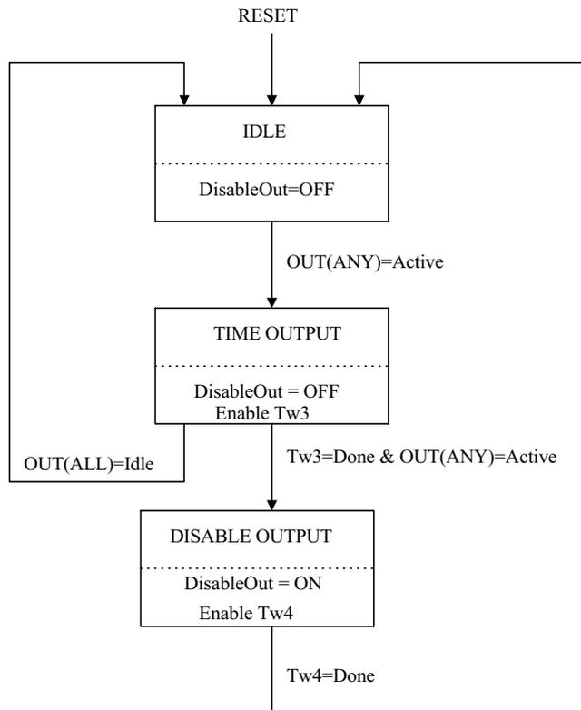
Figure 6. MAU jabber Lockup Protection State Diagram
