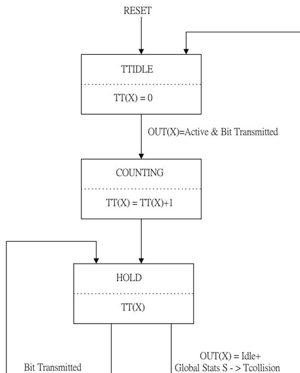
Figure 7. Transmit Timer State Diagram for Port X.
