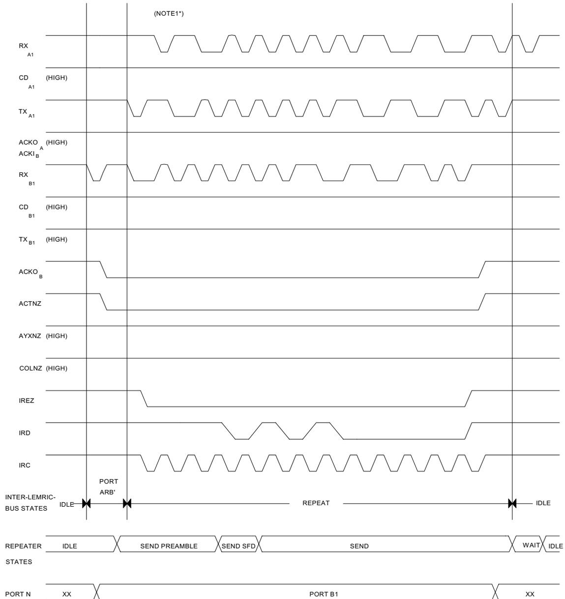
NOTE 1: The activity shown on RX<sub>A1</sub> represents the transmitted signal on TX<sub>A1</sub> after being looped back by the attached .
