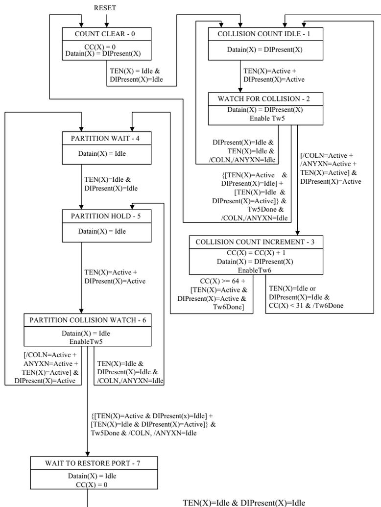
Figure 2. Partition State Diagram for TP Port X
