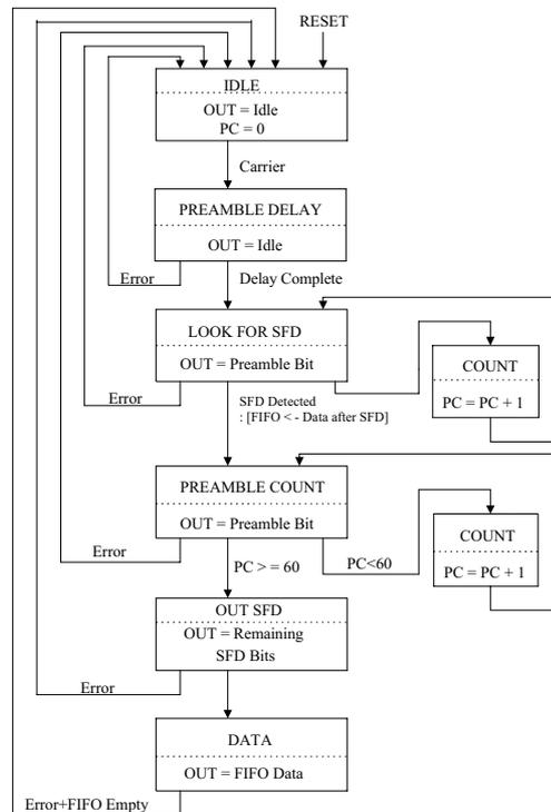
Figure 8. State Diagram for Automatic Preamble Regeneration
