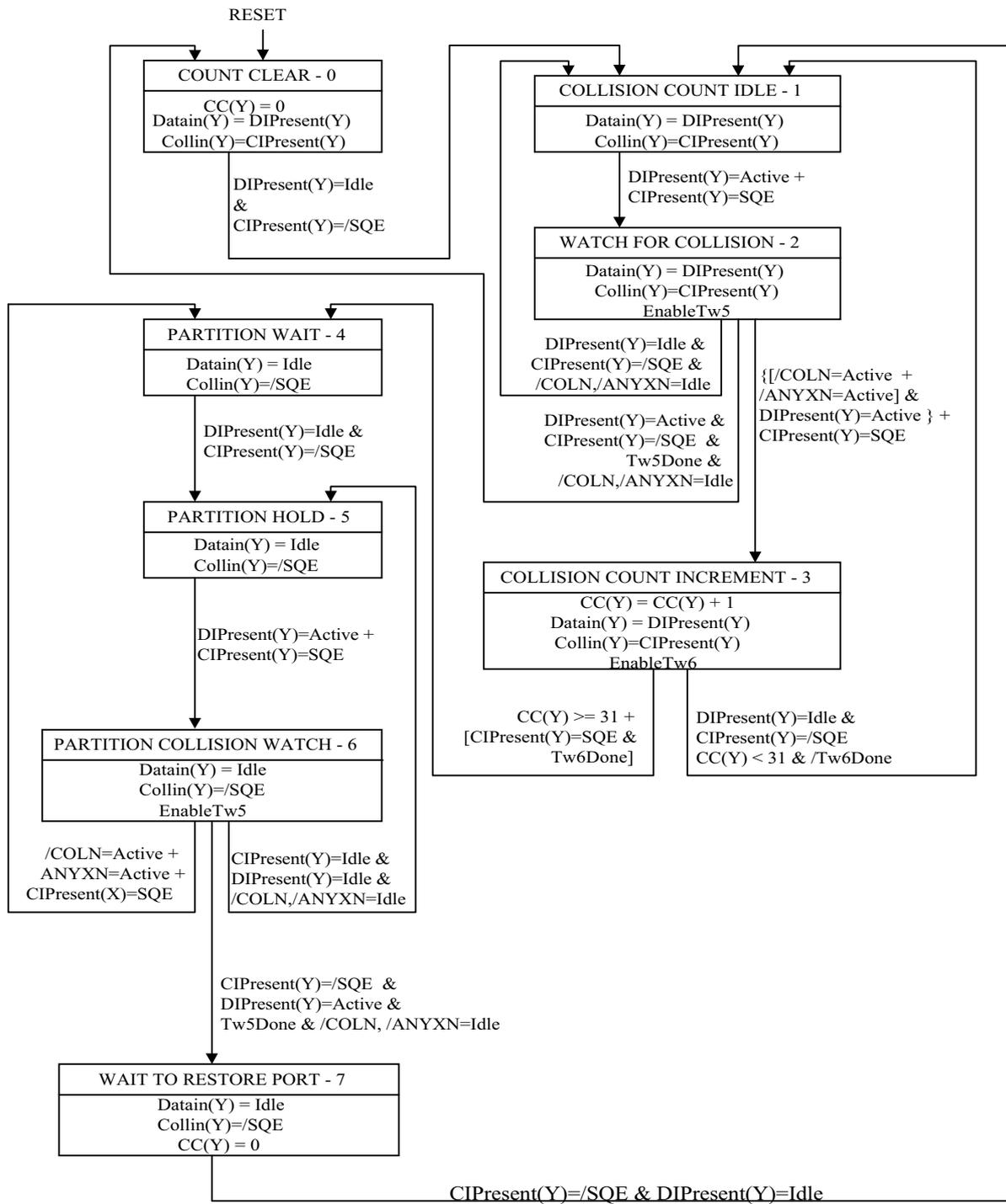
Figure 3. Partition State Diagram for AUI Port Y
