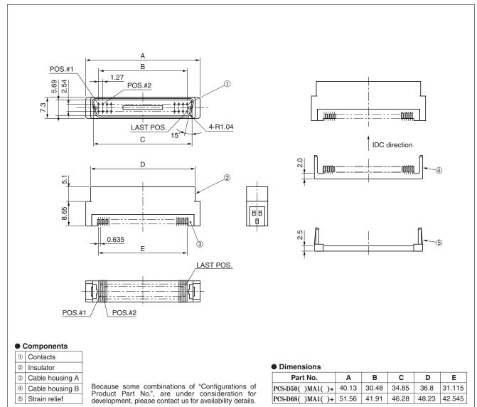
Mating connectors: PCS series straight through hole type female connector for PCB
