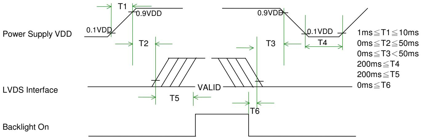
Apply the lamp voltage within the LCD operating range. When the backlight turns on before the LCD operation or the LCD turns off before the backlight turns off, the display may momentarily become abnormal.
