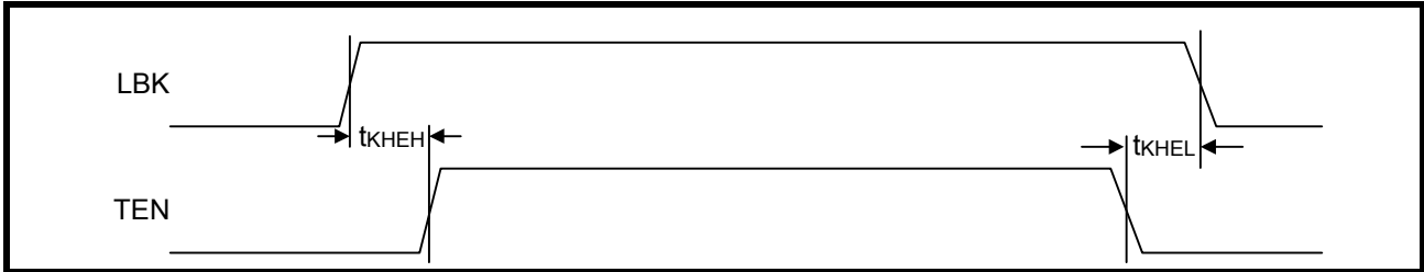
Figure 35: Mode 3 Loopback Timing
