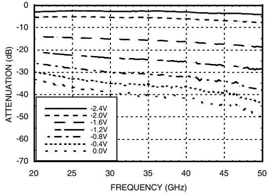
**Attenuation vs. Vctrl Over Temperature**
