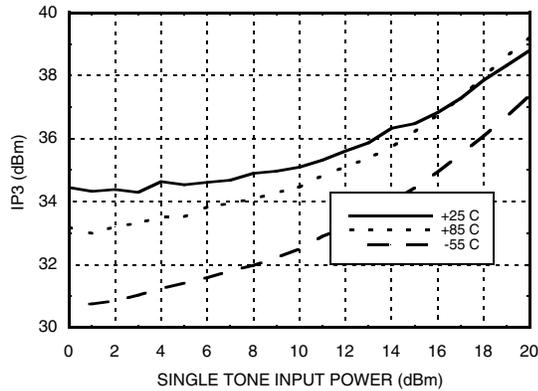
**Input IP3 vs. Input Power @ 30 GHz
