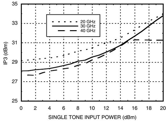
**Input IP3 vs. Input Power Over Temperature @ 30 GHz**
