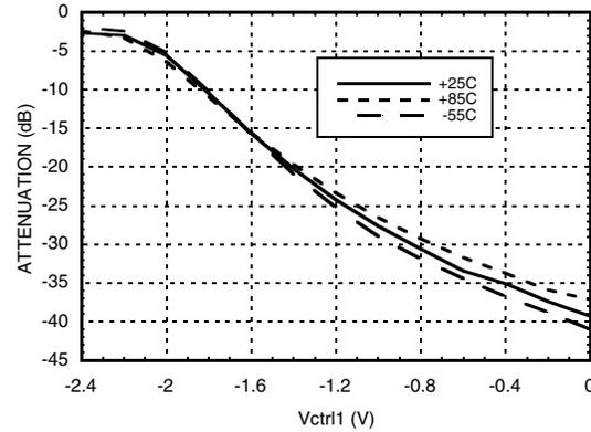
**Attenuation vs. Pin @ 30 GHz Over Vctrl**
