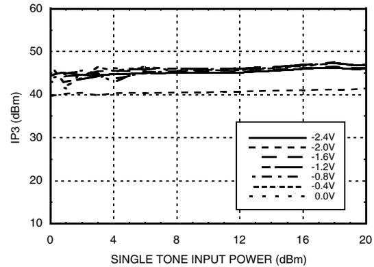
**Input IP3 vs. Input Power Over Frequency
