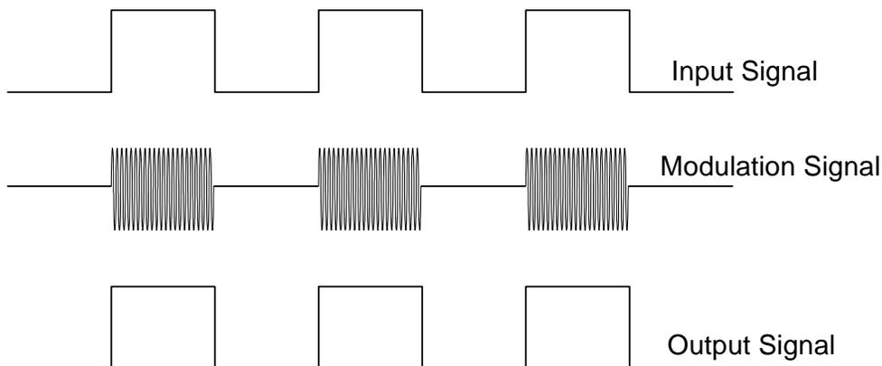
**Figure 10. Modulation Scheme**
