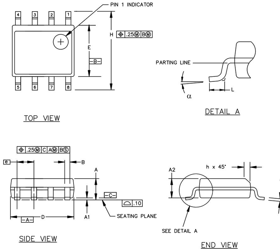
Figure 15. 8-pin Small Outline Integrated Circuit (SOIC) Package
