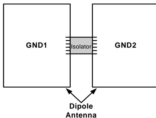
**Figure 13. Dipole Antenna**
