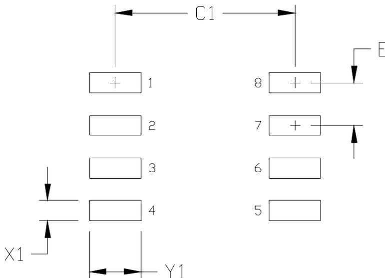
**Figure 16. PCB Landing Pattern: 8-Pin Narrow Body SOIC**
