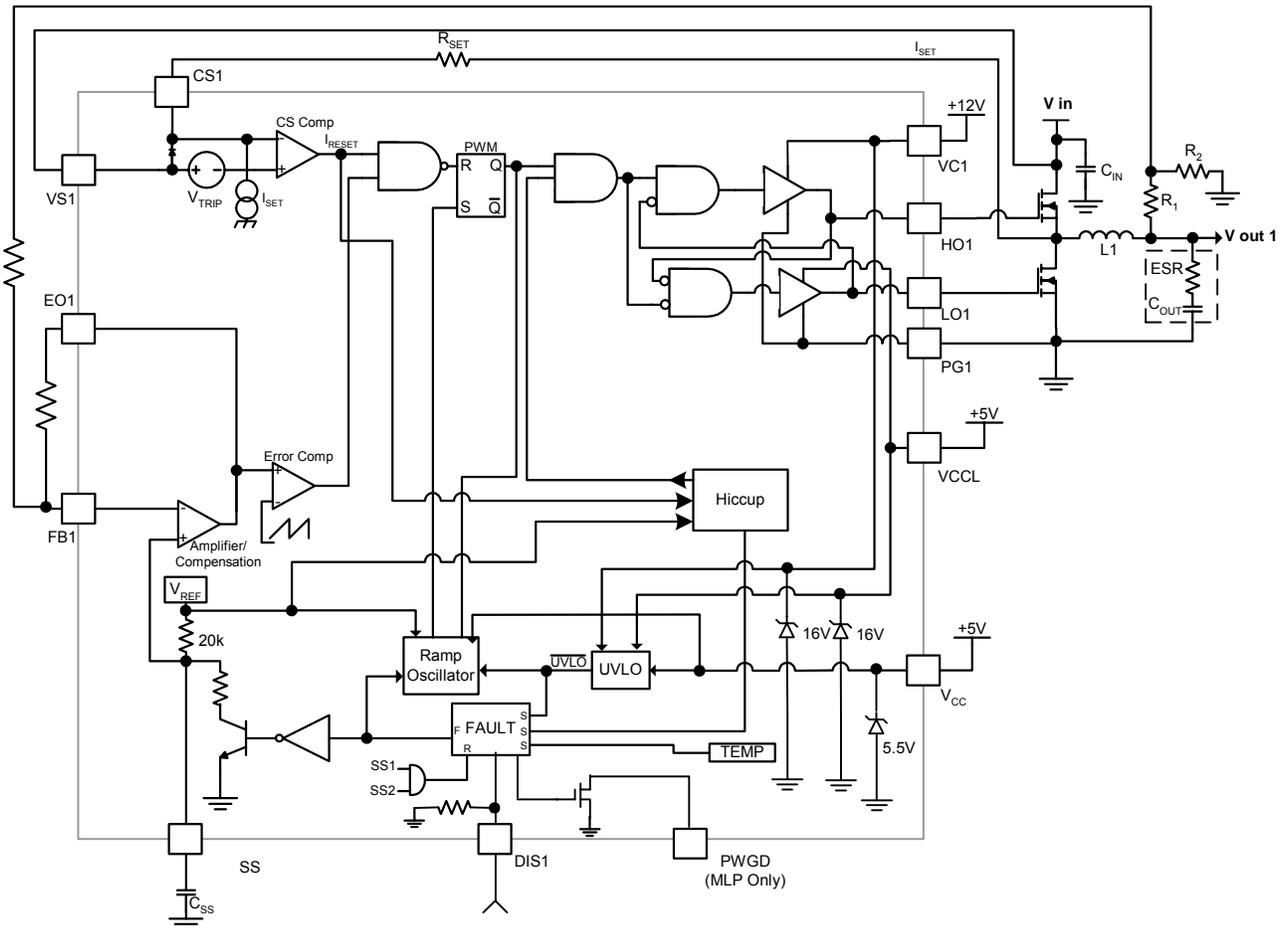
**Figure 1 – Block Diagram of PWM Phase 1**
