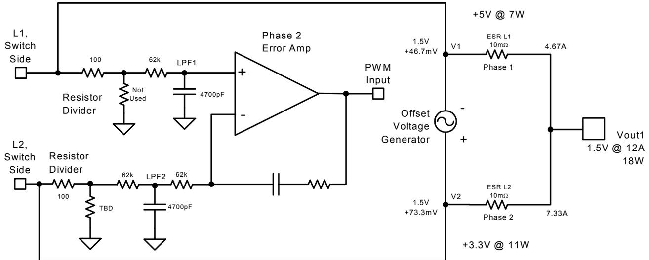
**Figure 8 – LoadSHARE Using Feedback Divider Offset**
