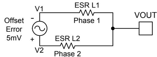
**Figure 6 – Error Amplitude**
