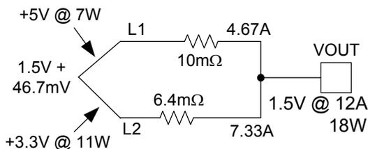
**Figure 7 – Ratio LoadSHARE Using Inductor ESR**
