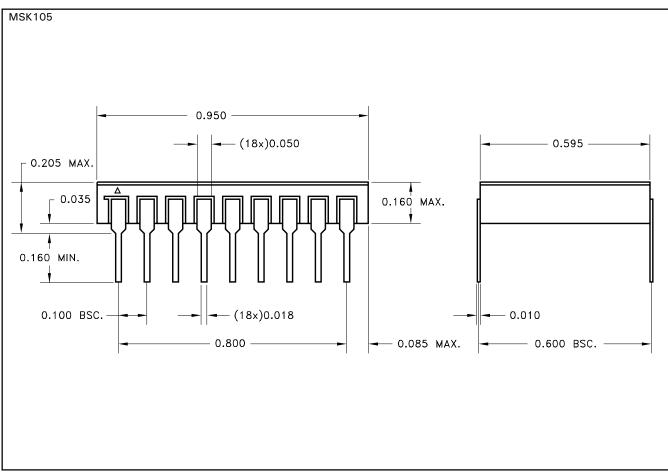
$\label{eq:solution} \begin{array}{c} \text{ESD TRIANGLE INDICATES PIN 1.} \\ \text{ALL DIMENSIONS ARE } \pm 0.010 \text{ INCHES UNLESS OTHERWISE LABELED.} \end{array}$
