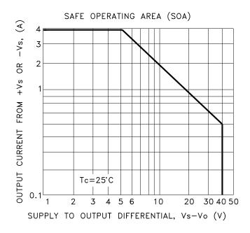
Safe operating area curves are a graphical representation of all of the power limiting factors involved in the output stage of an operational amplifier. Three major power limiting factors are; output transistor wire bond carrying capability, output transistor junction temperature and secondary breakdown effects. To see if your application is meeting or exceeding the limitations of the safe operating area curves, perform the following steps:
