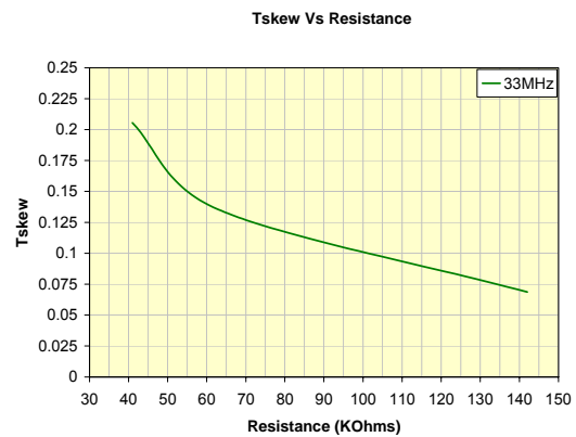
Fig6: Tskew Vs Resistance (33MHz, FS=0)
