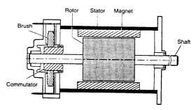
The stator is formed by a metal carcass and one or more magnets that create a permanent magnetic field inside the stator. At the rear of the stator are the brush mountings and the brush gear which provide electrical contact with the rotor.
