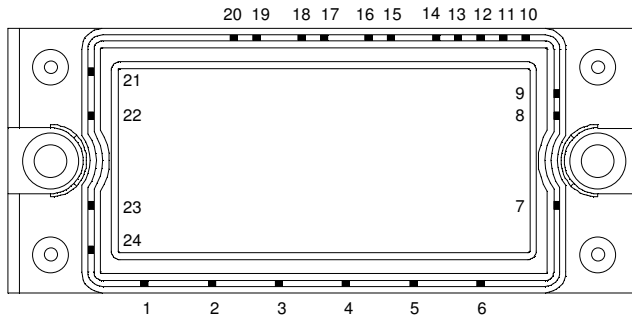
APTGS15X120RTP2: Without Brake (Pin 7 & 14 not connected)
