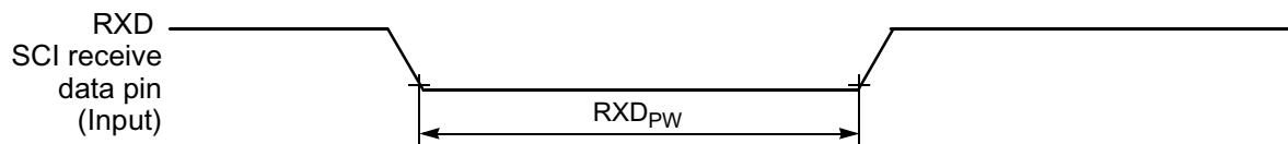
Figure 10-15 RXD Pulse Width
