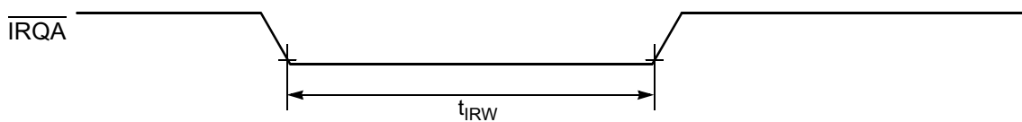
Figure 10-6 External Interrupt Timing (Negative Edge-Sensitive)
