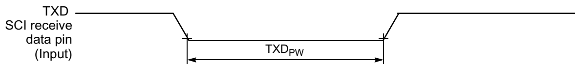
Figure 10-16 TXD Pulse Width
