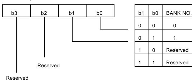
The Bank Select Reg. can select the active bank. The memory size of each bank is 512\*4 bits. Bank 0 and bank 1 are normal SRAM.
