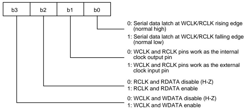
The serial interface configuration is shown below:
