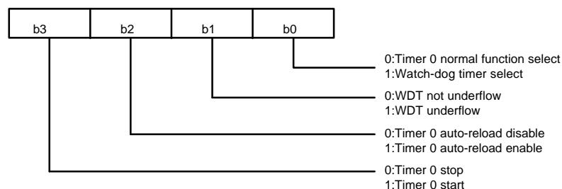
If Timer 0 works as a Watch Dog Timer, then bit1 of the STTM0 REG will be set when WDT underflows. Meanwhile, the system is reset just as in a power on reset except for the STTM0 bit1. The WDT (STTM0 bit1) will only be reset to zero during a power on reset or during the RAM write mode.
