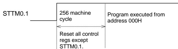
As watch dog timer underflows, the STTM0.1 is set, in the mean while, system and all control registers, except data 1 in STTM0.1 bit is reserved, are reset to initial state then after a delay of 256 machine cycle time program is executed from address 000H. After system reset, user can detect STTM0.1 to recognize which method of reset was done before.
