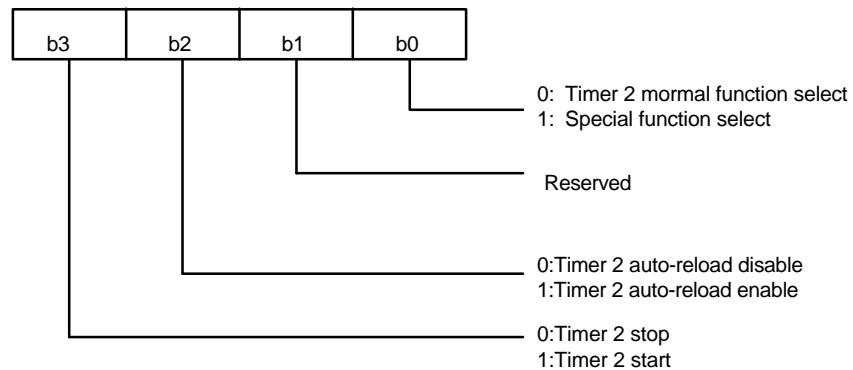
If Timer 2 is in the timer mode, the Timer 2 will underflow when it goes from 00H to FFH. The value in TM2MSB and TM2LSB will be auto reloaded to the Timer 2 Set REG. Timer 2 will decrease by 1 continuously at each clock transition after the timer has started.
