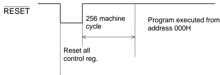
As RESET pin is pulled low, system and all control registers are reset to initial state. After RESET pin is in high level, system will delay 256 machine cycle time then program is executed from address 000H.
