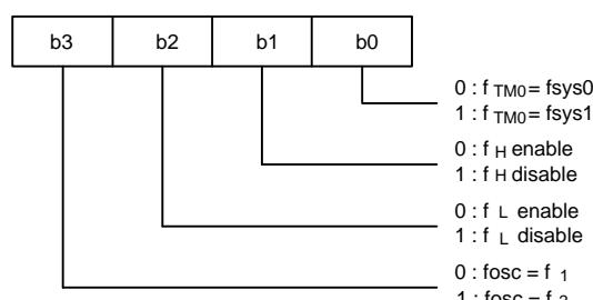
The W921E880A/W921C880 provides a crystal or RC oscillation circuit selected by bit0 of the INI register (refer to 6.14 INITIAL CONDITION Section) to generate the system clock through external connections. If a crystal oscillator is used, a crystal or ceramic resonator must be connected to OSCI and OSCO, and the capacitor must be connected if an accurate frequency is needed. The oscillator configuration is shown as follows.
