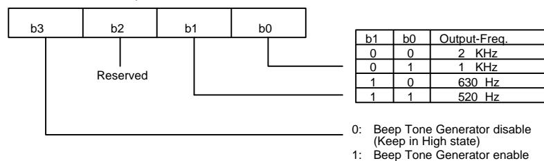
If the Beep Tone Generator is disabled by setting the BTGR REG. bit3 to "0" or after a power on reset, the BTG output pin will remain in a high state.
