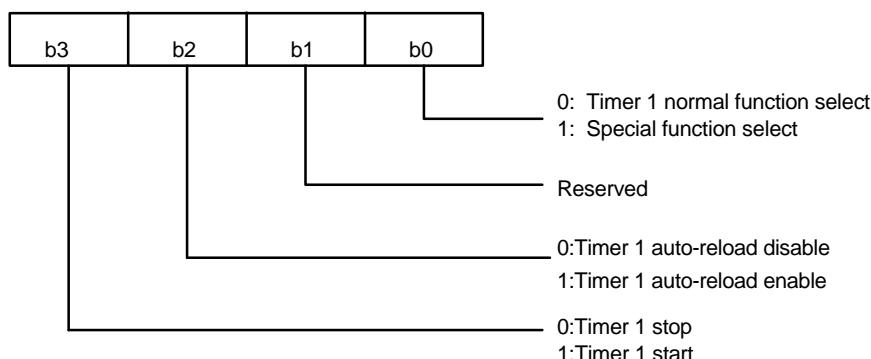
If Timer 1 is in the timer mode, the Timer 1 will underflow when it goes from 00H to 0FFH. The value in the TM1MSB and TM1LSB will be auto reloaded to the Timer 1 Set REG. when the STTM1 bit2 is set. Timer 1 will decrease by 1 continuously at each clock transition after the timer has started.
