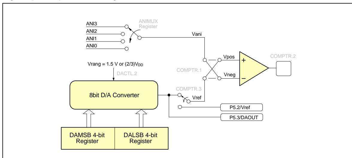
ù D/A Converter Control Register:
