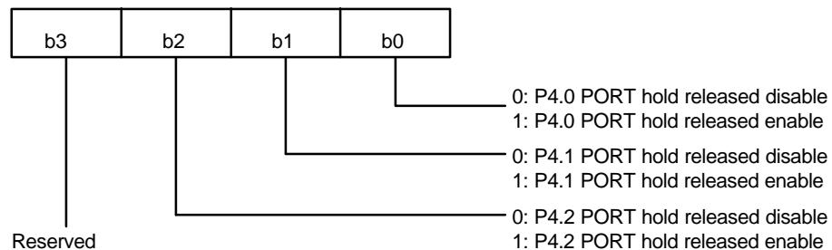
The HOLD RELEASED STATUS FLAG 1, 2, 3 (HRSTS1, 2, 3) (ADDRESS = 03CH, 03DH, 03EH) stores the information that caused the HOLD MODE to be released. The format is shown below.
